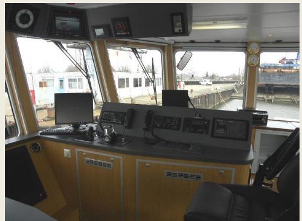
SB Forward bridge console
