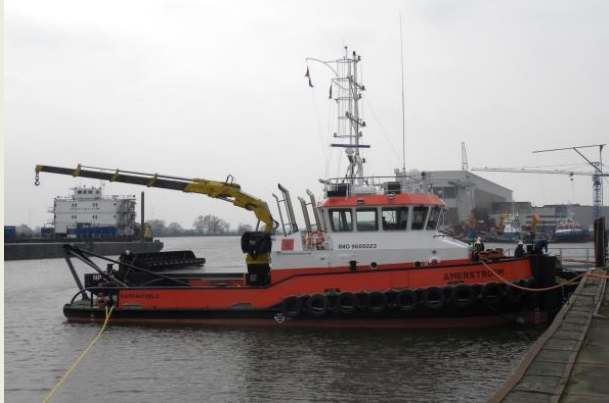
Eurotug 2300 with crane in full length
