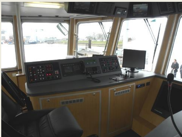
PS forward bridge console
