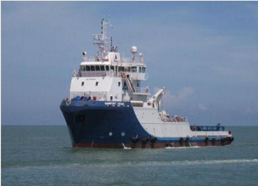
that is represented by the innovative firm. The first of the two vessels, the **Mainport Cedar**, has now been delivered while the sister-ship **Mainport Pine** will deliver later this year. Wartsila Ship Design of Singapore designed the 54.6 by 13.8-meter seismic support vessels. Main engines for the vessels are a pair of Cummins QSK60M-MCRS IMO Tier II. Each engine produces 2200 BHP at 1800 RPM and turns a four-blade Berg Propulsion controllable pitch propeller
