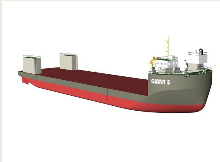
Submersible draught aft is 17.0mtrs.; submersible draught fwd is 17.0mtrs and grounding draught aft is 20.0m. The Singapore registered pontoons are classed Lloyds Register +100 A1 Pontoon, Submersible to a maximum draught of 17m, IWS, WDL (20t/m<sup>2</sup>). They are available in the Far East as from autumn 2014. The vessels will be built at Nantong; China.
