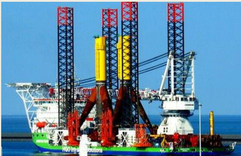
Last week was seen the *HLJV Innovation* of HGO Infrasea Solution sailing out from Eemshaven after loading two no's Tri pods weighing each 900 T and 6 no's monopoles. She is sailing out to Global Tech 1 Windfarm. *(Photo: Mohan Divakaran-Sr Jacking Engr of JB 117)*
