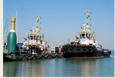
standby." The tugs have a bollard pull of 62.5 tons and a speed of 13.5 knots. (Photo: Richard Wisse)
