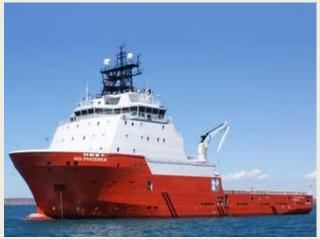
Norwegian designed and DNV classed, **Go Phoenix** is a highly complex *VS 491* 24,000 bhp Anchor Handling Tug Supply vessel with a hybrid propulsion diesel electric drive. It is DP 2 and FiFi 2 capable, delivering up to 260 t of bollard pull. Otto Marine's first 24,000 bhp vessel is deployed in the Asia Pacific region and recently completed the rigmove of one of the largest rigs in the region for an oil major. *(Source: Otto Marine)*
