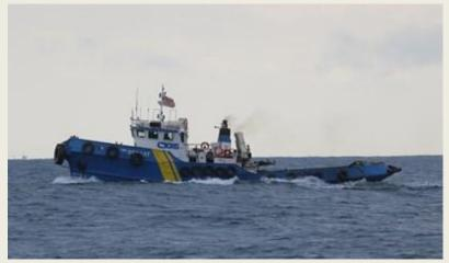
draft of 3.08 mtrs. The Crepelle main engine develops an output of 1,150 at 1,800 rpm. The 126 grt and 34 nrt tug has a max speed of 10 knots and a bollard pull of 15 tons. Further the tug is equipped
