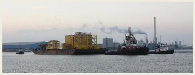
One day later 11<sup>th</sup> August was seen the departure of the Accommodation module and helideck for the above DolWin Alpha platform loaded on the Heerema barge H-302. The leading tug for the transport is the **Bugsier 9** from Bugsier Reederei. Assistance during the river transport was given by the Muller Dordrecht tugs **En Avant 7** at the bow; **En Avant 4** and **Sirius** at the stern. *(Photo: Willem Holtkamp)*
