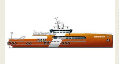
Incat Crowther has been contracted to design a trio of 42.5m Monohull Dive Support Vessels. The design is an innovative new concept borne of the latest ideas from designer, builder and operator. The design has been developed from stem to stern to be a dedicated DP-2 capable Dive Support Vessel, featuring fully integrated ROV launch and recovery, dive compressors and decompression chamber. The
