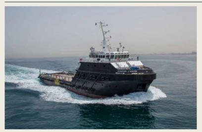
Grandweld has completed the delivery of a new vessel that will be used in firefighting on offshore platforms. **Stanford Hunter**, a 57meter Offshore/Maintenance vessel bought by Stanford Marine, will help with maintenance and firefighting on offshore platforms on a 24-hour basis. The vessel can accommodate 50 crew and comes with two powerful 1450KW CAT engines that can produce a speed of 13.5 knots. For fast deck-cargo
