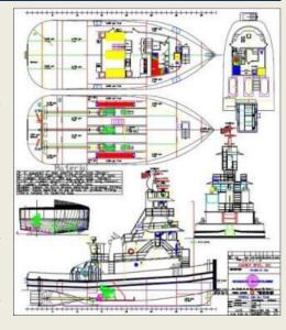
making up to barges. Work in and around the shallows of the Mississippi deltas and bayous can present real challenges to a tug that must also navigate sections of open water. With nearly 2000 HP, this vessel from Rodriguez will add to the shipyard's well-established reputation for tugs designed and built with deep draft power in a shallow draft tug. General Arrangement courtesy of Rodriguez Shipyard. (Source: Alan Haig-Brown)
