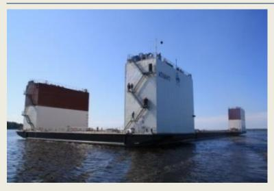
Vyborg Shipyard completed on July 29 two-day sea trials of a semisubmersible heavy-lift barge "Atlant", the company said on Tuesday. The shipbuilder's trials included a series of tests of the vessel's systems and its performance during submersion and refloating. On August 5 the barge will be put into service and become a dock platform for fabrication of the 21900M-class icebreaker's hull. Vyborg Shipyard is part of the stateowned United Shipbuilding Corp.
