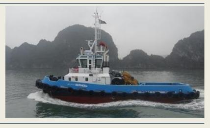
Caterpillar 3512C TA/C develops a total output of 2,460 bkW (3,300 bhp). She achieved 46,3 ton bollard pull and a speed of 12.3 knots. The tug is classed Bureau Veritas I X HULL • MACH Tug Unrestricted Navigation incl. loadline and tonnage certificate. (Source: Damen)
