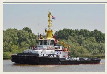
LEADING towage and salvage specialist Multraship has further strengthened its multipurpose fleet with the addition of the ASD tug Multratug 20. Multraship has contracted with international broker and consultant DSB Offshore for the long-term bareboat charter of the 72-ton bollard-pull vessel, which was built by the Bogazici Shipyard in Turkey in 2010 and is equipped to undertake a range of services including towage, escort, anchor-handling, firefighting and salvage. Multratrug 20 has
