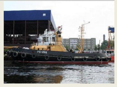
objects, oil and petroleum content products, cargo transportation, ice breaking and erosion operations. *Technical information* Length max 25,4 m; Width max 8,8 m; Draught 4,2 m. Speed 11,8 knots; Bollard pull 23 tonnes. Classificaion KM Arc4 R3 Aut3 Tug by Russian Maritime Register of shipping. Propulsion system Z-drives US 155, Rolls-Royce, FPP into nozzles. Powerplant 2x746 kW at 1800 r/min, Caterpillar C32. *Deck equipment:* •bow electro-hydraulic anchor-towing-mooring
