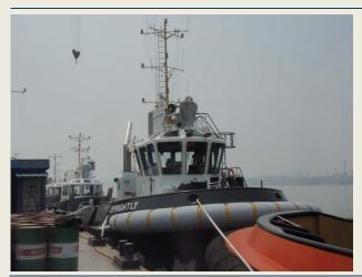
On the Damen Shipyards Changde was seen the Damen ASD 2009 tug **Springthly** fitting out upon delivery. The tug will sail to Darwin (Australia). A standard ASD 2009 has a length of 21.19 mtrs a beam of 9.43 mtrs. The total engine output is 1,940 bkW. They have a speed of 11.2 knots and a bollard pull of 30 tonnes (*Photo: Clemens Smits ©*)
