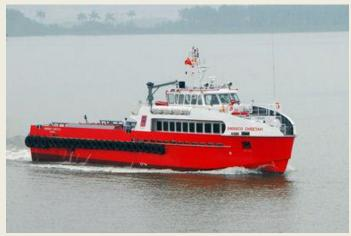
tankage includes 57,400 liters of fuel and 21,250 liters of fresh water. Accommodation is provided for ten crewmembers in six cabins and seating for up to 70 passengers. Forward doors in the deck cabin permit the option of transferring personnel from the bow. The Cummins Hong Kong branch supplied the three Cummins KTA38-M3 HD engines that power the Swissco Cheetah. Each engine delivers 1007 kW (1350 bhp) at 1900 RPM to fixed-pitch propellers
