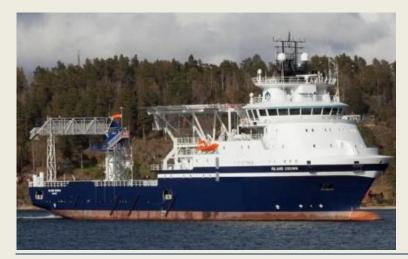
is outfitted for offshore Inspections, Maintenance and **Repairs** addition to general subsea work. Vessel equipment includes a longreach offshore crane and permanent heave compensated gangway system for safe and easy access to and from offshore installations. (Source: Island Offshore)
