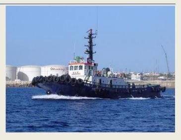
Her speed is 13.6 knots and the bollard pull 47 tonnes. The grt is 185 tonnes and dwt 89 tonnes.
