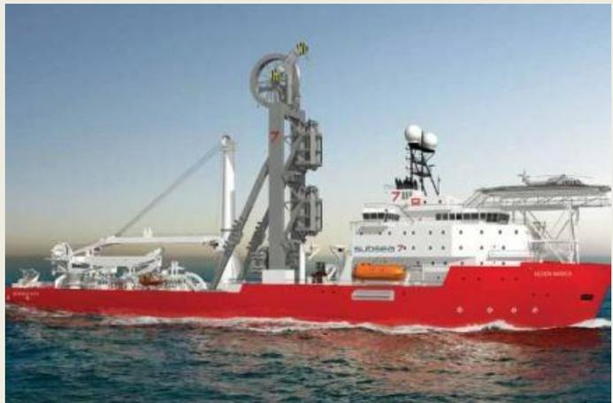
globally to meet increasing market demands for executing ever-larger and more complex projects. She will have 2,600m<sup>2</sup> deck area (for equipment carriage), a 600t Active Heave Compensated offshore crane, a 325t top tension vertical lay system and a 7,000t under-deck basket for storage of flexible pipes, umbilicals and cables. The vessel will be equipped with six main engines in two engine rooms designed to maximise performance in Dynamic Positioning Class III. *(Press Release)*
