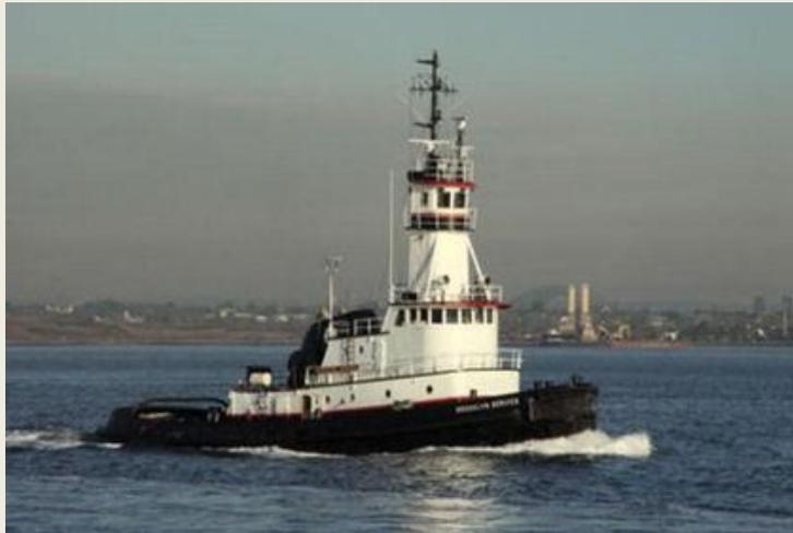
speeds of abt. 8.5 – 10kn. Although laid-up at the time of the sale, both tugs were still actively classed ABS +A1, Towing Service, +AMS, Unrestricted Service. Each tug is fitted with a single drum Markey TDS-32 towing winch with a capacity of 2,000' of 2" wire. Other features include raised pilot houses and air conditioned quarters for 10 crew aboard each boat. New owners plan to reactivate both tugs under U.S. flag for use in their in-house service. Marcon acted as sole
