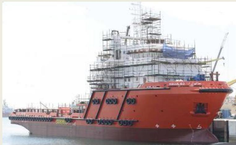
classed for unrestricted service, and is equipped with Dynamic Positioning capability of DP2. She is powered by two 2,720KW MAN Engines, and is fitted with two controllable pitch propellers, two stern thrusters, and two bow thrusters. The vessel is scheduled for delivery end of July 2013. Principal particulars: Length Overall: 67 meters; Breadth: 16.80 meters; Depth: 6.80 meters; Draft, loaded: 5.40 meters; Bollard Pull: 90 Tons; Speed: 13.5 knots; Complement: 50 Persons. *(Source: Grandweld)*
