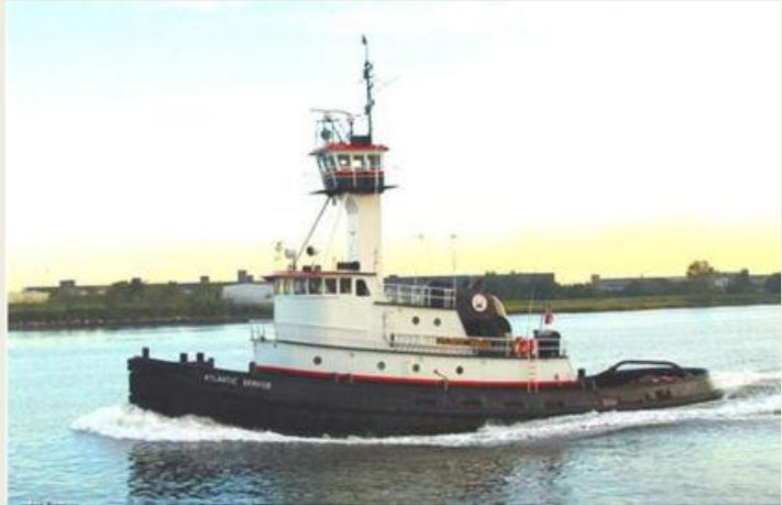
and Amerada Hess Corp. of New York until the Hess fleet was acquired by Leevac Marine / Hornbeck. The tugs measure 109' length overall x 31' beam x 14' depth. Both "**Atlantic Service**" and the "**Brooklyn Service**" are powered by twin EMD 16-645E2 main engines, Falk gears and 4-blade 100" x 76" high-efficiency props, which develops bollard pull of about 34.5 tons and free running
