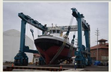
Cleveland, Ohio. Great Lakes Shipyard continues to make progress on the construction of two tugboats for SEACOR Holdings, Inc.'s new Aura Class. Hull 9201 was the first of the tugs to be launched using the Shipyard's 770-ton Travelift. The tugs will undergo various testing over the upcoming weeks. Great Lakes Shipyard was awarded contracts by Caribbean Tugz, LLC, an affiliate of SEACOR Holdings, Inc., to simultaneously build the new state-of-
