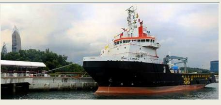
anchor handling, rig support and supply and standby operations. With over 11,900kW, the vessel is fitted with DP2 dynamic positioning and is "well equipped for the challenges of the offshore oil and gas industry". Mr Tan Ser Giam, managing director of the Eastern Navigation group, commented:
