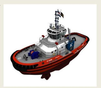
bollard pull of 80 tons. KOTUG needed an additional powerful harbour tug quickly and Damen could deliver her from stock".
