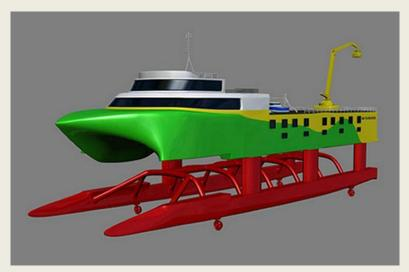
with its new patents pending design making it the only vessel on the world capable of transforming from a high speed catamaran to a semi-submersible platform. This innovation has enormous global potential for use in the offshore energy markets, such as platform personnel transfers and wind farm maintenance, offshore survey, inspection and installation works. The patents pending Submersible Hull Vessel (SHV TM) concept is owned by OSSeas Ltd and is the
