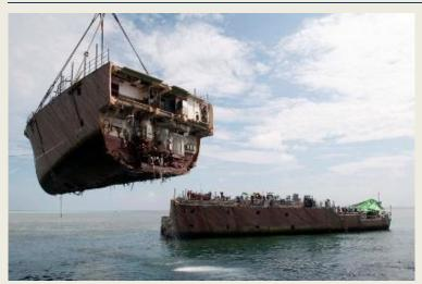
U.S. Navy and contracted salvage personnel embarked aboard M/V Jascon 25 have begun dismantling and sectioning the hull of the grounded mine countermeasures ship Ex-Guardian. The bow section was safely lifted and removed from Tubbataha Reef to an awaiting barge, March 26. This work has been accomplished in close coordination with the Philippine Coast Guard, Philippine Navy, and Tubbataha Reefs Natural Park. The remaining
