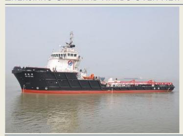
Zhenjiang Shipyard successfully delivered, on March 22nd 2013, the 10,000 kW multi-purpose Offshore Supply Vessel named **Xing Yun Yang** to Nanjing Sumec Shipping Co. The vessel is equipped with DP2 automation and can meet the requirements of Unattended Machinery Space (UMS) in unrestricted area. (Source: Zhenjiang Shipyard)
