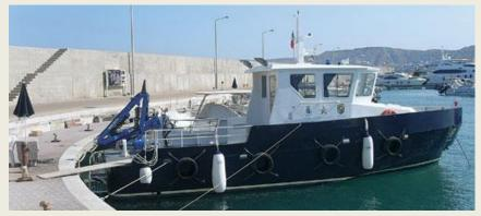
Rizzuto, near Crotone in South Italy. The boat is used to transport technical staff (up to 12 people and three crew), as well as monitoring, positioning, rescue, and patrol of the MPA. A multi-purpose boat for a range of duties, the work boat/survey vessel
