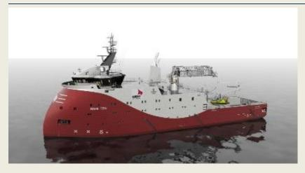
The "Siem Moxie", an infield support vessel (ISV), will be put into operation in spring 2014. She is the first work boat with the Ulstein-designed X-BOW to be fitted with two Voith Schneider Propellers (VSP). X-BOW vessels are characterised by the absence of a bulbous bow. Their bow slopes backwards above the water line which results in
