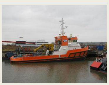
two Mitsubhi S12U-MPTK main engines develops a total output of 4,410 kW. It is expect that she achieved a board pull during trails of 83 tons. He is classed Bureau Veritas with notation  $I \neq Hull \bullet$  Mach Unrestricted navigation AUT-UMS; Ice class 1A super. *(Photo: Piet van Roon)*
