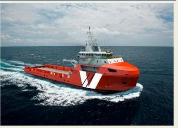
subsea-support vessels on order. *Vessel Particulars (not guaranteed)* Length overall (approx.) 78 m; Breadth moulded 18.4 m; Depth to main deck 7.8 m; Max. draught / Design draught 6.0 m; Deadweight at max. draught 3,600 tonnes Special Class Notation (ABS) DPS-2, FiFi 1, UWILD, Enviro. Deck load 1,500 tonnes; Cargo deck area 750 sqm. Gross / Net tonnage international 2,950 / 895. Max. speed 13.0 knots. Additional information MLC2006 and SPS2008 compliant, Green Passport. *(Source: Vroon)*
