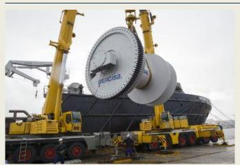
Ibercisa delivers the first of two towing winches AHT type model MR-E/930/2/2500-89 which will be installed on the Anchor Boat (AHT) "Bylgia" which Hereema Marine Contractors from Holland have signed with the Armon shipyard in Vigo. The electrically driven winch is the first of its kind in the world to be given this drive which has meant quite a challenging technological feat for the Vigo based Company given the dimensions and characteristics of the machine. The "Bylgia"
