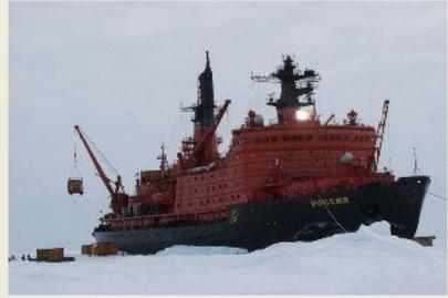
The Rossiya is the third in the Arktika-class of Russian nuclear icebreakers. It was launched in 1985 and is the oldest of the four remaining active heavy nuclear icebreakers in the Russian fleet. There are also two shallow-draft nuclear icebreakers that work primarily on northern rivers. The **Rossiva** (which means "Russia" in Russian) displaces 23,000 tonnes and is powered by two OK-900 reactors. It is normally used to escort vessels
