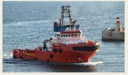
The 2011 built Italian registered with call sign IIXR2, 10,800hp anchor handling tug Almisan (Imo 9553581) entering Grand Harbour, Malta on Sunday 3rd March, 2013 for the first time bound to Palumbo Malta Shipyard Ltd.The AHT is owned and managed by Augusta Offshore SpA. - Naples; Italy. She has a grt of 1,659 tonnes and a dwt of 1,264 tonnes and is classed
