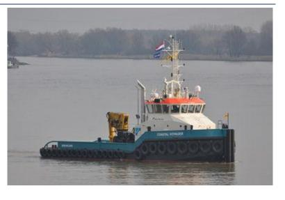
the tug during the trails she achieved a bollard pull of 48 tons and a speed of 11.5 knots. The basic functions of the tug are Towing, mooring, pushing, anchor handling, dredging support operations.
