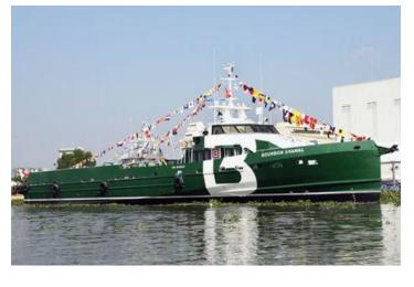
length. Through this investment, Piriou asserts its determination to produce in series this type of ships at competitive price and high quality. **Bourbon Shamal** is a 53m FSIV, the largest of Piriou Inhouse designed FPSV comprehensive range, which includes vessels from 19m to 53m. (*Source: Piriou*)
