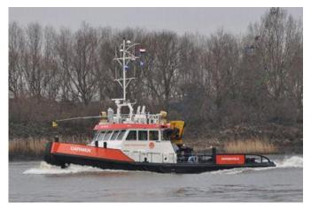
will working for the Tym-Group. The tug with yard number 571623 was built in Poland and fitted out at the Damen Shipyards Hardinxveld: Netherlands. She has a length 23.35 mtrs a beam of 8.00 mtrs and a depth at sides of 2.99 mtrs. She has a displacement of 238 tons. Her basic functions are Towing, mooring, pushing, anchor handling, dredge support operations. The two Caterpillar 3412D TTA develops a total output of 1,264 bkW (1,696 bhp). She achieved 24.1 ton bollard pull ahead and
