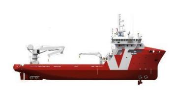
both passengers and crew. She is scheduled for delivery in early 2015 and will be operated by Vroon Offshore Services B.V. in Den Helder. *Vessel particulars (not guaranteed):* Length o.a. - 68 m; Beam - 14.95 m; Special Class Notations (ABS). Greenpassport, Enviro, SPS, MLC 2006, DP Class, Class 2, ABS. Accommodation Total of 50. *(Source: Vroon)*
