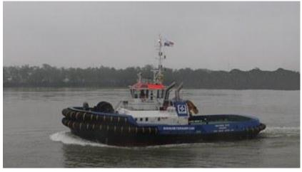
functions are Push-pull, escorting, towing and fire fighting operations. The two Caterpillar 3516C HD+TA/D develops a total output of 5,050 bkW (6,772 bhp). She achieved 76.5 ton bollard pull ahead and 72.9 ton astern and a speed of 14.6 knots ahead and 14.4 to astern. The tug is classed Lloyds Register of Shipping. (*Source: Damen*)
