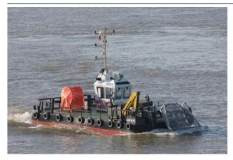
The Multicat 1506 **Sirius** was recently delivered to her owners Tuapse Commercial Sea Port (TCSP) - Russia. The Multicat with yard number 517511 was built on the Damen Shipyard Gorinchem; China. She has a length 15.50 mtrs a beam of 6.06 mtrs and a depth at sides of 2.25 mtrs. Her basic functions are Debris collecting, pollution control and bilgewater collecting. The two Volvo 5DA TA/2 develops a total output of 236 bkW (320 bhp). She achieved a bollard pull of 2.7 tons
