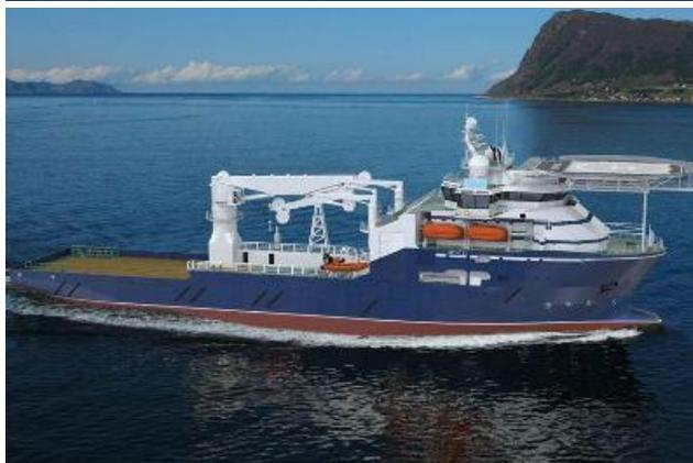
Rem Offshore ASA has entered into a long term contract agreement with an international company for the subsea support and construction vessel “**Rem Installer**”. The vessel, MT 6022 design from Marin Teknikk, will be delivered from Kleven Verft AS in June 2013. Among its features will be a powerful offshore crane able to lift 250 tonnes at 650 metres or 135 tonnes at 3000 metres water depth. The firm contract period is 3 years, with an option for charterer to change the fixed period to 5
