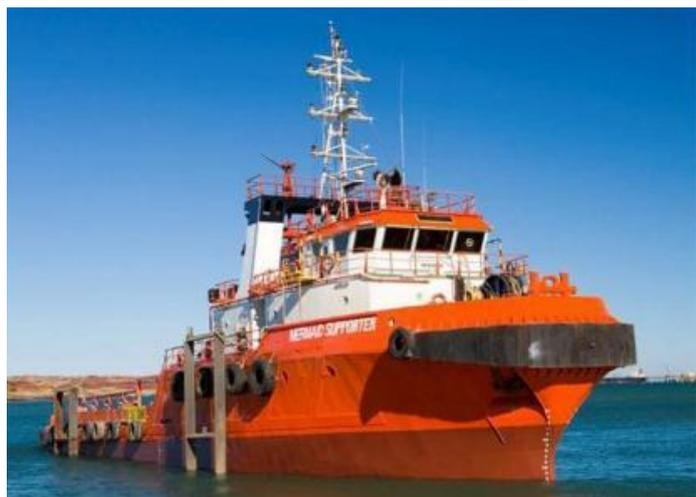
The contract is for an initial period of five years, with contract upside should the two additional one year options be exercised by the Company. The **Mermaid Cove** is a 53m DP2 Offshore Support Vessel (OSV) and a sister ship to the 53m **Mermaid Strait** and 50m **Mermaid Sound**. These two sister vessels are on long term contract with Woodside. The **Mermaid Cove** shares design features with her sister vessels that enable her to work in close quarters operations to tankers
